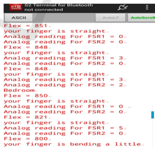
Figure 3: Sensor readings as shown in the smart phone.
