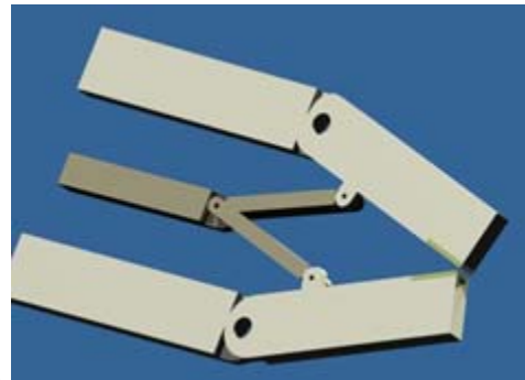
Figure 3: Designed scissors mechanism.
