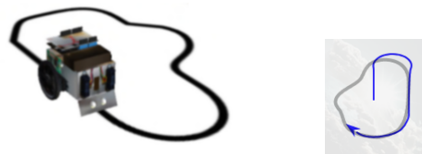
Figure 2: The Line Follower robot (INTO-CPS project http://projects.au.dk/into-cps/ ) and an example of a robot trajectory.
