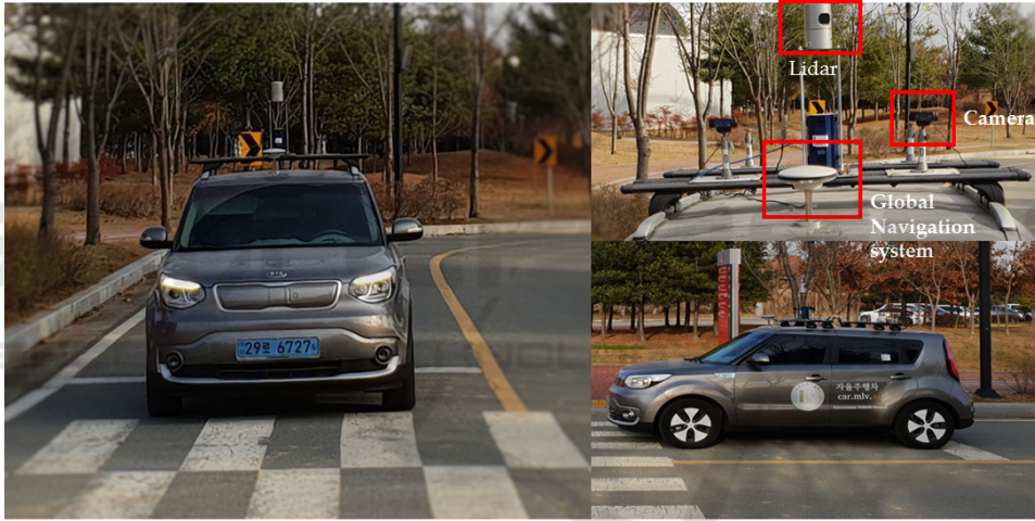
Figure 2: MLV-Self Driving Car KIA Soul EV equipped with different sensors being used for collecting the data.
