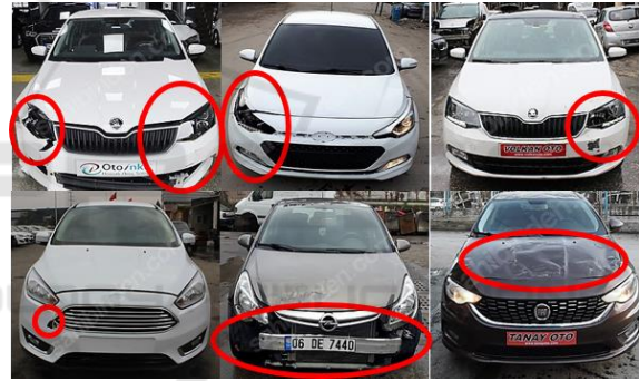
Figure 8: Sample damaged vehicle images from the test set with red ellipses enclosing the ground truth damaged areas. The first row shows samples successfully classified as damaged. The second row shows incorrectly classified damaged vehicle samples.
