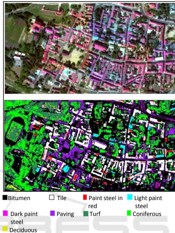
Figure 5: Recognition based on the spectral database of urban materials (roof, human-made, vegetation).
