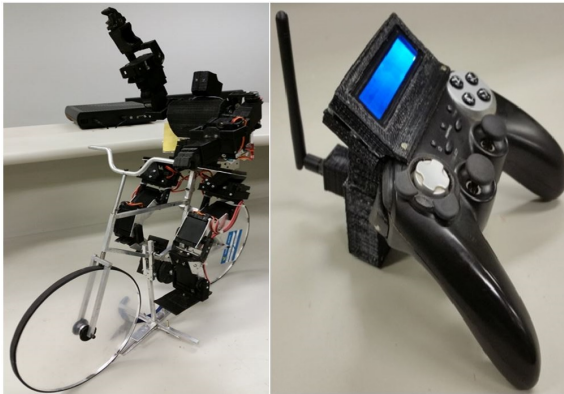
Figure 7: Assembled robot (second prototype) and joystick remote control.
