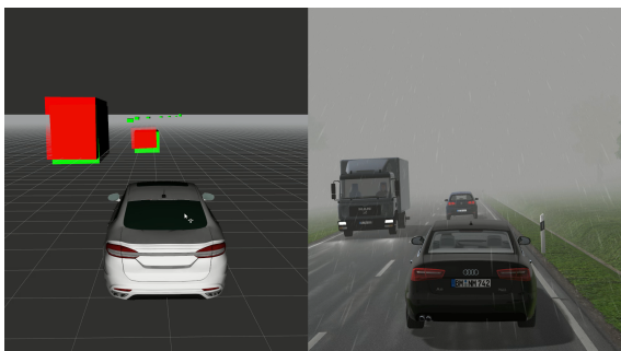
Figure 5: Visualization of OSI objects in ROS (Left) in comparison to VTD (Right), undetected objects are marked as green, detected as red.
