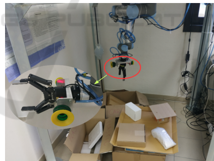
Figure 1: Robotic recycling system using a multifunctional grasping tool.
