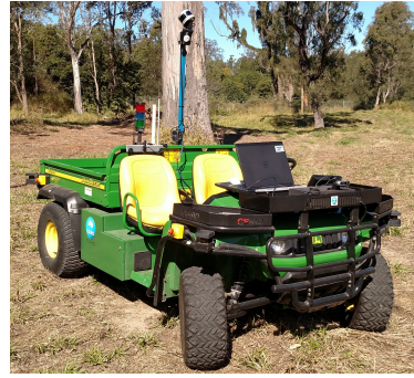
Figure 4: The robot used, a John Deere Gator holding multiple sensors.
