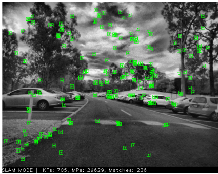
Figure 5: Sample image after the Adaptive Histogram Equalization, the green dots stands for the detected ORB features.
