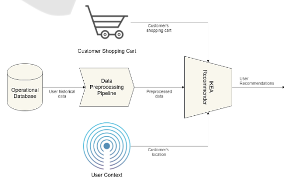
Figure 2: Recommendation engine conceptual diagram. Data are retrieved by the operational database and fed to the data pre-processing unit. In real-time the customer's location and shopping cart are fed as extra input to the model, to create an incremental context-aware recommendation engine.
