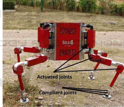
Figure 1: A leg of SILO4 walking robot (Gonzales et al, 2003) showing its various active and passive joints.
