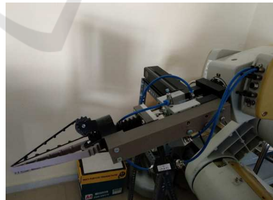
Figure 6: Gripper of the robotic system.
