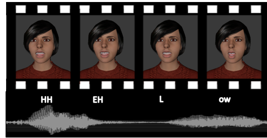
Figure 3: A film strip of an animated character. The avatar is controlled by control points. These controls are of two types, facial controls and the body rig. Examples of a facial controls include mouth-open, left-brow-right-up, left-brow-mid-down and mouth-right-corner-up. Examples of body rigs include neck, left-eye-lid, jaw and spine.
