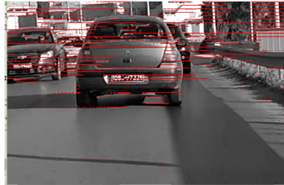
Figure 1: Optical flow vectors calculated with Horn and Schunck Method.
