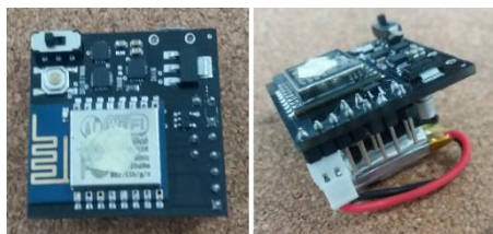
Figure 5: IMU Sensor with battery and ESP module.
