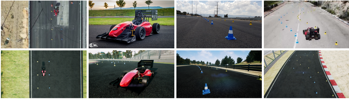
Figure 2: Images taken from our simulated environment (bottom) and from real tracks we have driven in (top). The simulation was built to have objects resemble their real-world counterparts precisely, including the exact traffic cones and our Formula SAE car. Both the real world and the simulated environments consisted of straight and swerved tracks as shown. Our model was trained in simulation only and was executed in a real-world environment.
