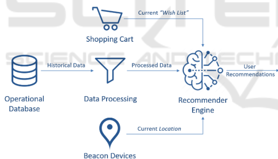
Figure 1: IKEA skip gram context-aware recommender conceptual diagram. Data are retrieved by the operational database and fed to the neural network through the data pre-processing unit. In real-time the customer's location and shopping cart are fed as extra input to the model.
