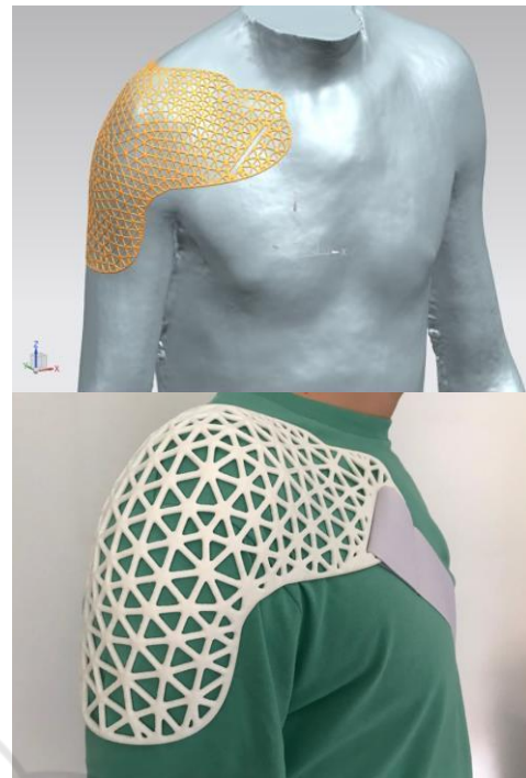
Figure 1: Personalized design and 3D printed prototype of a shoulder splint for injured joint immobilization. Designer: Eduardo Martínez. Collaborator: Marina Maestro. Mentor: Andrés Díaz Lantada.
