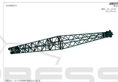
Fig 5. Finite element model of 13m main arm.
