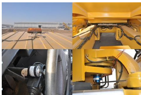
Figure 6. Sensor installation position.
