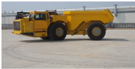
Figure 5. Testing field of 35 tons electric drive underground articulated mining truck.
