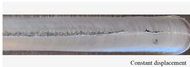
Figure 7. Weld formation of constant displacement.
