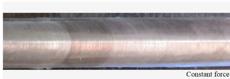
Figure 8. Weld formation of constant force.
