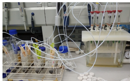
Figure 2: Soil supernatant was flowed through SPE cartridge for absorbing metsulfuron methyl.
