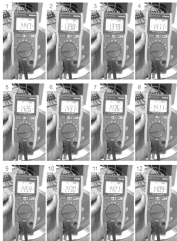
Figure 16: Battery Current Data Acquisition with Solar power plant
