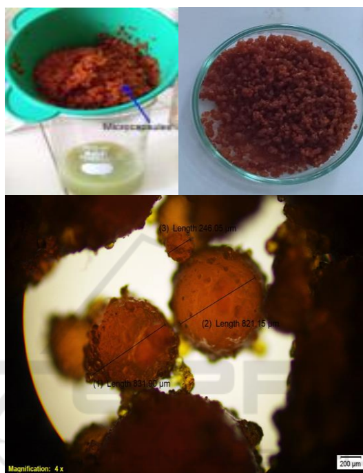
Figure 3: The morphology of clove oil microcapsule in a polyurethane shell.
