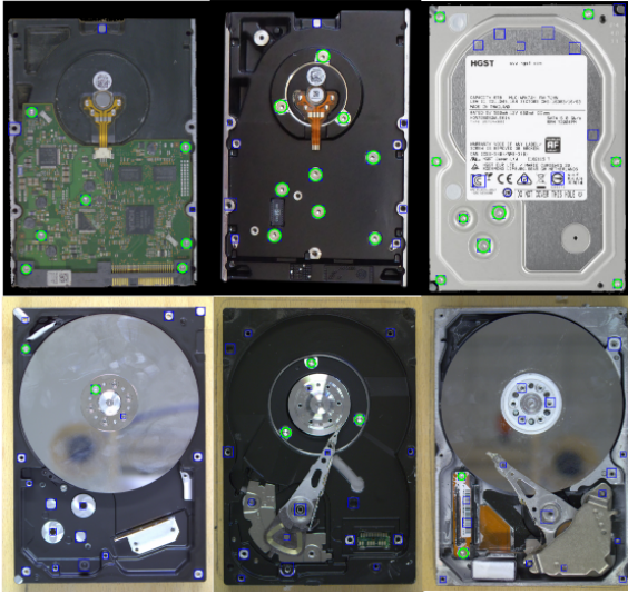
Figure 4: Outputs from the integrated screw detection module. Blue circles highlight the candidates suggested by the Hough circle finder, whereas green circles are the detected screws by the model taken from a study (Yildiz and Wörgöter, 2019).
