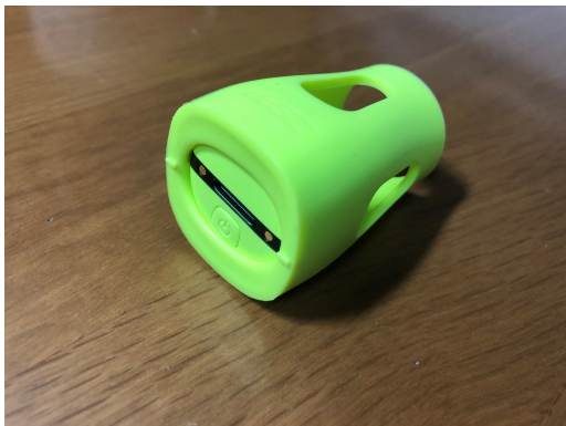
Figure 1: Smartsensor can be attached to the grip end of the racket and can measure the rotation direction, speed, rotational speed, etc. of the stroke.
