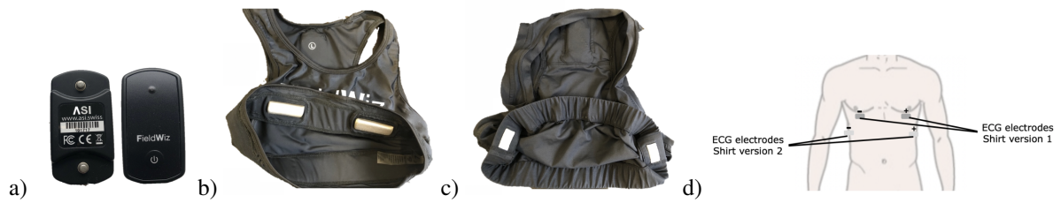
Figure 2: Experimental acquisition setup. (a) FieldWiz device; (b) Wiz connected Shirt, Version 1; (c) Wiz connected Shirt, Version 2; and (d) Electrodes placement for both shirt versions (FieldWiz, 2020).
