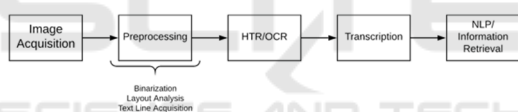
Figure 1: The steps in a conventional HDP workflow for handwritten and printed documents.
