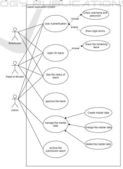
Figure 2: Use case design for leave management system.
