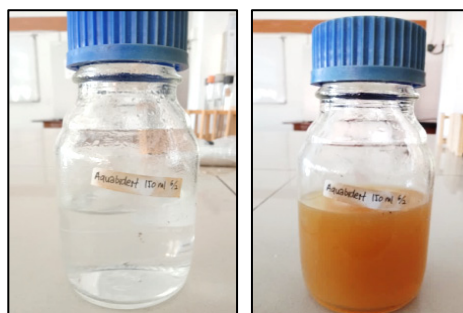
Figure 1: AgNO 3 solution before the synthesis process (left) and LL-AgNP after the synthesis process (right).
