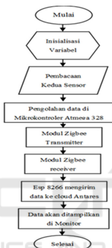
Figure 3.2. Software Design Flow Chart
