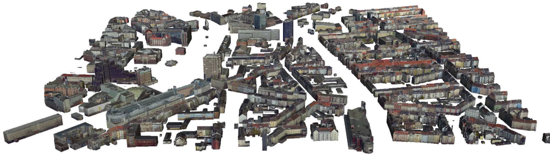
Figure 5: Test data: Our variant of RANSAC was used to estimate roof facets of this model of a square kilometer of the city of Dortmund.
