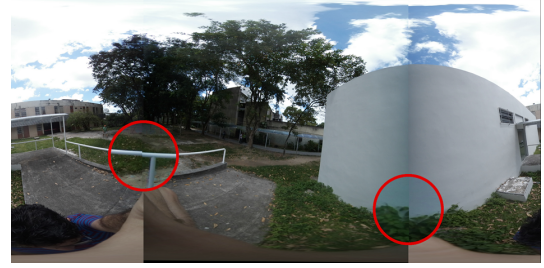
Figure 2: Although the global alignment is adequate in most of the image, it is possible to note artifacts on specific regions (red circles).
