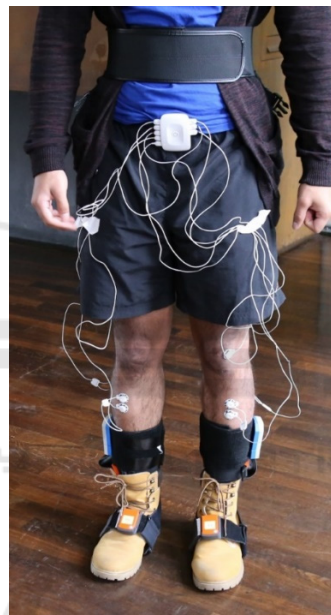
Figure 1: Experimental setup – Xsens and PLUX sensors are applied.
