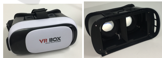
Figure 5: Head-mounted displays utilized in our experiments. (Right) This HMD device has a divider between two lenses, so subjects could easily perform the parallel-eyed stereo method.
