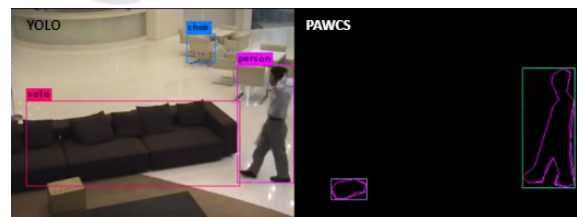
Figure 2: Debug output example of the sofa scene: Left: YOLOv3 (threshold:0.5). Right: PAWCS. The box is detected only by PAWCS, the sofa and chair only by YOLO.
