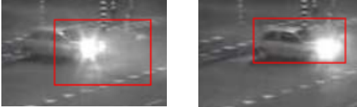
Figure 7: Frames from street scene. Left: Car was only detected by BGS. Right: Car detected by YOLO.
