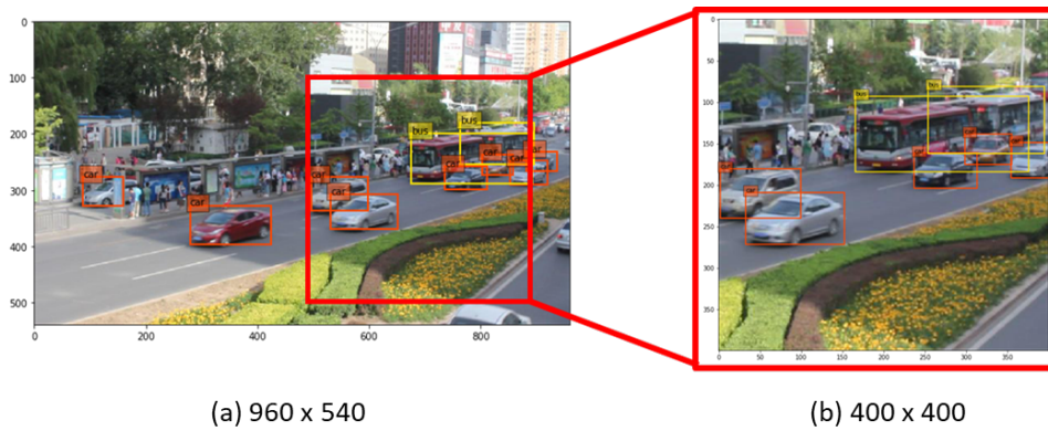
Figure 3: Detection results of FSSSD with input size (a) 960 \times 540 and (b) 400 \times 400 .
