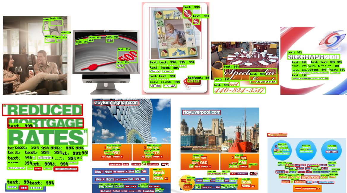
Figure 7: Examples of success (first row) and failure (second row) cases of the proposed approach for the ICDAR'11 dataset. Green bounding boxes indicate the regions correctly localized (true positives cases), while red bounding boxes show candidate regions were not detected by our method (false negatives cases).
