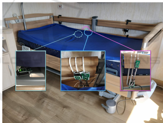
Figure 2: Picture of the sensor module at the care bed, including the Accel 5 click (left), the Weather click and Air quality click (middle) and Temp&Hum 2 click (right).
