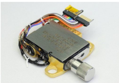
Figure 2: Flight Model of Raman Laser Module.
