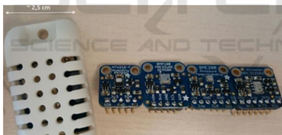
Figure 2: Low-cost sensors selected for the experiment. From left to right: AM2302, HTU21D, BMP180, BME280 and MPL3115A2.
