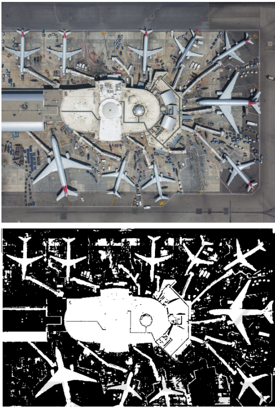
Figure 1: Symmetrical and asymmetrical objects in the airport image. Above is the original photo, below is the binary image obtained as a result of segmentation.
