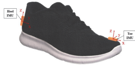
Figure 1: Schematic illustration of the position of the IMU sensors used in the proposed algorithm, including the three local axes (X-axis, Y-axis, and Z-axis). The two sensors are placed on the right shoe at the level of the first distal phalange (toe) and at the calcaneus (heel).
