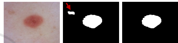
Figure 8: Image ISIC_0000092, left, the binarized saliency map where the only non-kernel component is pointed by the arrow, middle, and the result after the assignment of the non-kernel component to the background, right.
