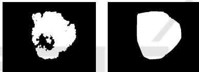
Figure 7: Saliency map at the end of the iterated binarization, left, and after pixels with lower saliency but adequate color have been assigned to the foreground, right.
