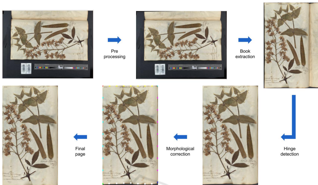
Figure 2: The proposed page detection pipeline.
