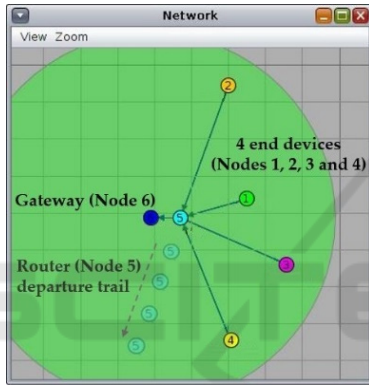
Figure 8: Simulation of network consisting of a (departing) mobile router and four end devices within Cooja.
