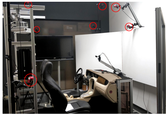
Figure 2: Driving simulator at our lab. The red circles highlights some of the motion capture system cameras.
