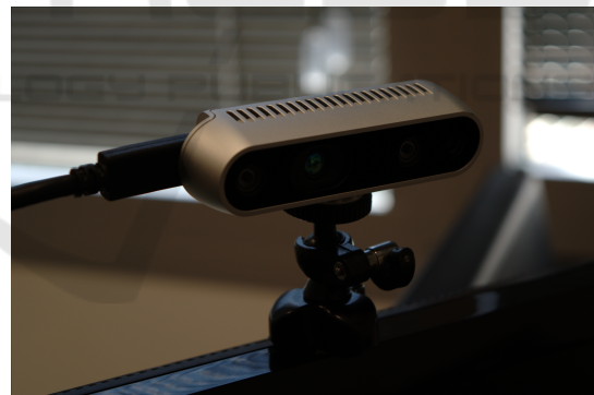
Figure 3: RealSense D435 Depth Camera for the Study of Facial Expression Located on the Top of the Perceptive Desktop Monitor.
