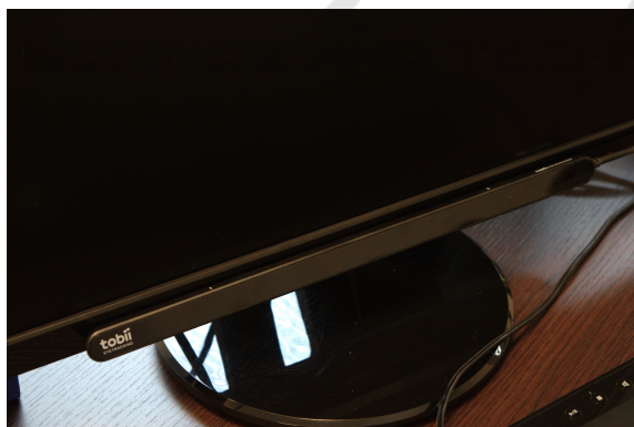
Figure 4: Eye Tracking Tobii 4c to Do the Eye-Tracking Study Located in the Lower Frame of the Perceptive Desktop Monitor.
