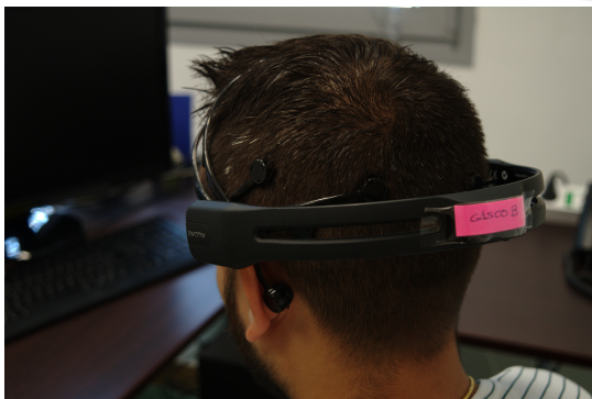
Figure 2: Emotiv EPOC Electrode Helmet for the Study of Brain Electrical Activity or Electroencephalography.
