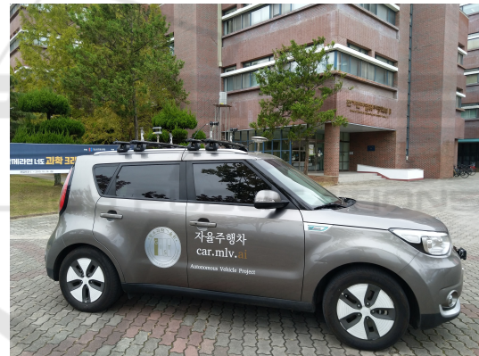
Figure 1: Our Self-Driving Car Equipped with State-of-the-Art Sensors That Includes Lidar, IMU, GNSS, Camera and Radar.
